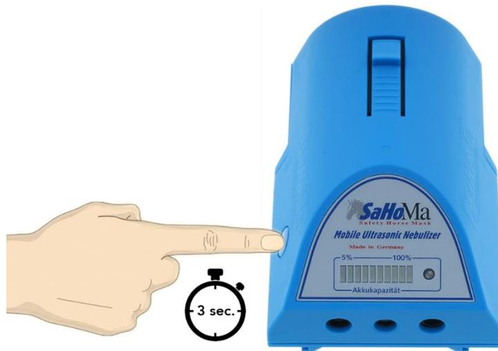
Immediately after starting, the light bar runs from left to right, the multifunctional light lights up green permanently and the nebulization starts in program 1.
